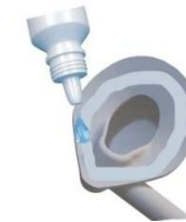
Figure 2: Apply Adhesive Around the Inside Rim of the Urine Collection Device Cup
